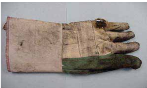
Figure 1. Glove damaged by leaking torch
